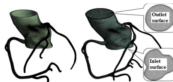
(a) domain meshes of the solid structure and the flow channel
