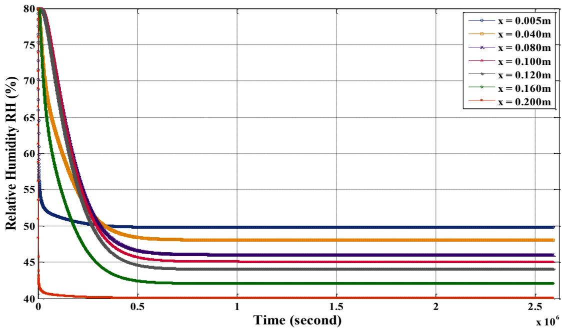
Figure 4. Temporal evolution of moisture at different abscissa of the wall for a pore radius of 0.001 nm.
