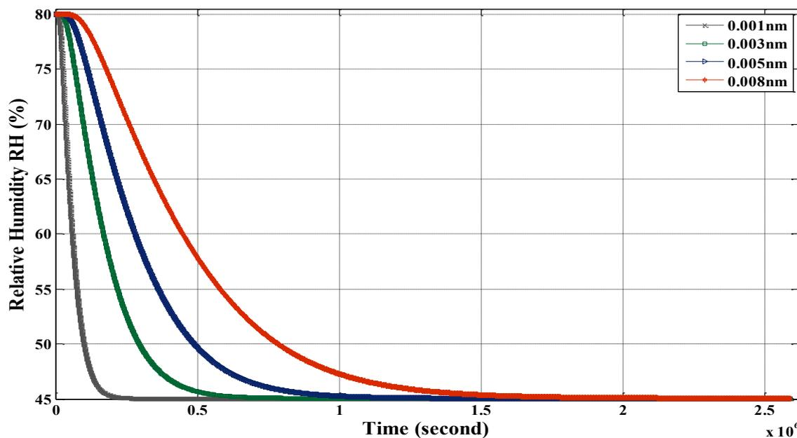
**Figure 5.** Temporal evolution of moisture in the middle of the wall, for different pores radius, 0.001 nm (black curve), 0.003 nm (green curve), 0.005 nm (blue curve) and 0.008 nm (red curve).
