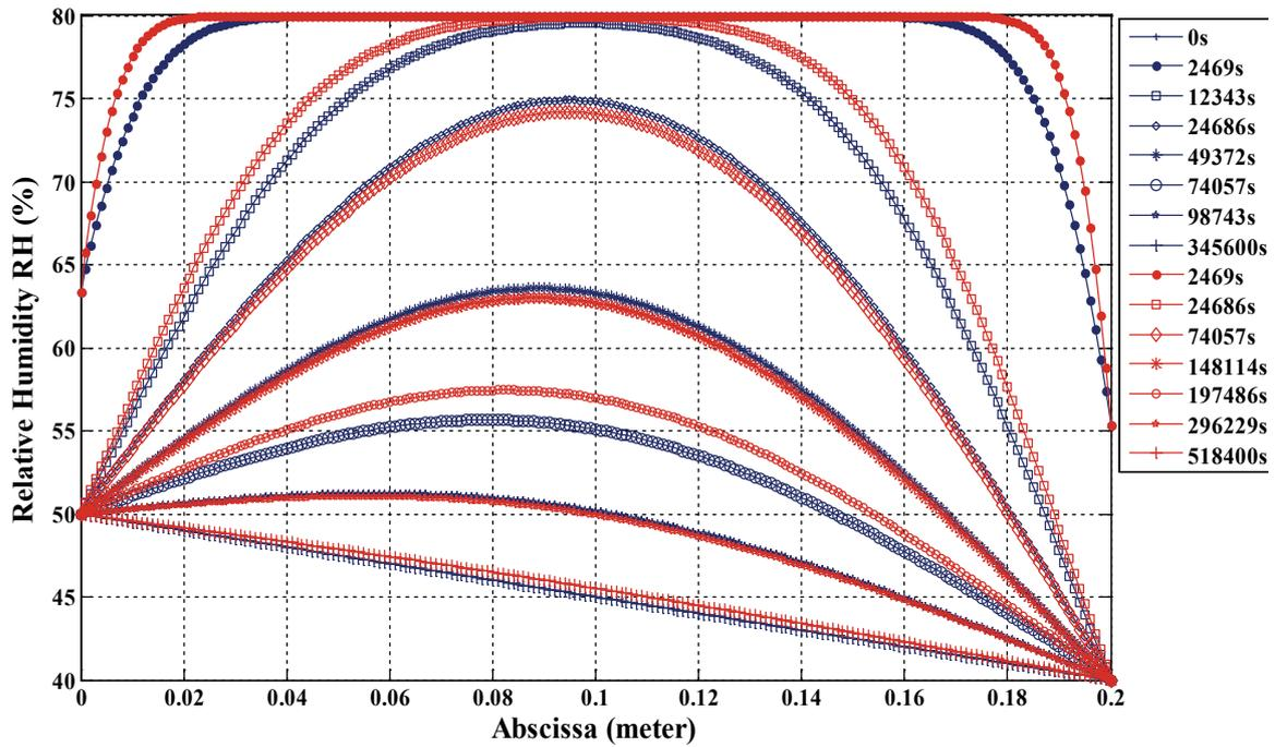
Figure 3. Spatial evolution of moisture at different times of simulation, for different pores sizes: 0.003 nm (red curves), 0.001 nm (blue curves).
