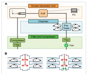
**Figure 1: Panel A:** Schematic of the nose-only, flow-past inhalation exposure chamber system. **Panel B:** Schematic of the tobacco exposure system. This system can remove the exhaled smoke and suppresses the effect of secondhand smoke (right).
