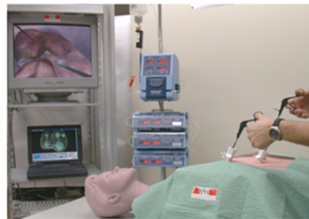
Figure 1: Surgical simulator with haptic feedback (Robotic Systems Laboratory LSRO).
