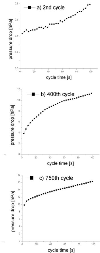
Figure 11. Pressure drop increase versus cycle time for an aging test with 2.5 m/min filtration velocity and 100 s cycle time
