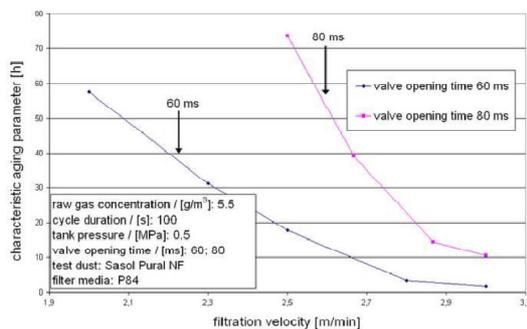
Figure 15. Characteristic aging line for different filter media
