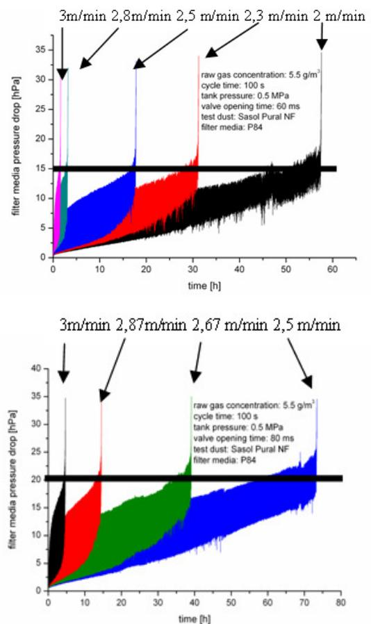
Figure 9. Aging test with different filtration velocities and two valve opening times
