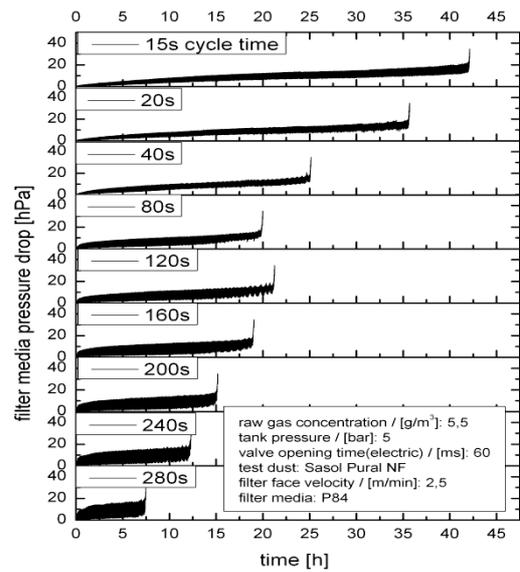
Figure 8. Pressure drop behaviour during the aging procedure for different cycle times [9]
