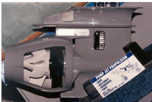
Figure 4: Pump jet propulsion system.
