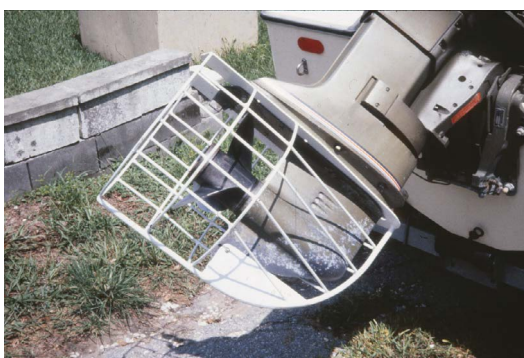
Figure 5: Cage type propeller guard.
