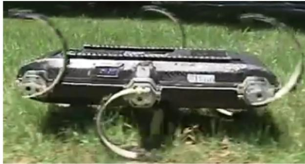
Figure 13: The RHex robot with the supporting legs at their tips P<sub>2</sub> (Courtesy of UPenn).
