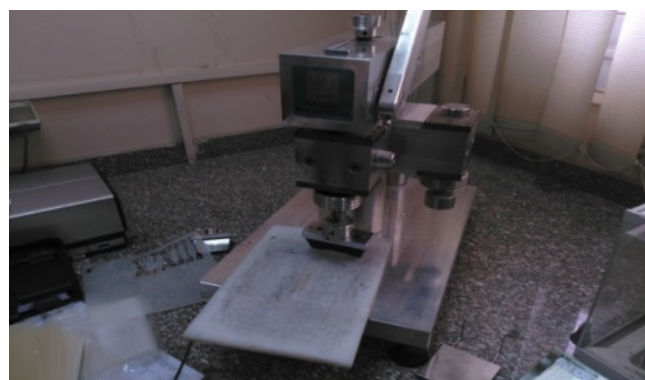
Figure 3: Dumbbell shape cutter instrument, according to ISO-527.
