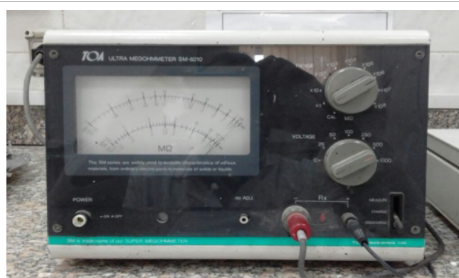
Figure 5: Volume resistivity tester ASTM-D275.
