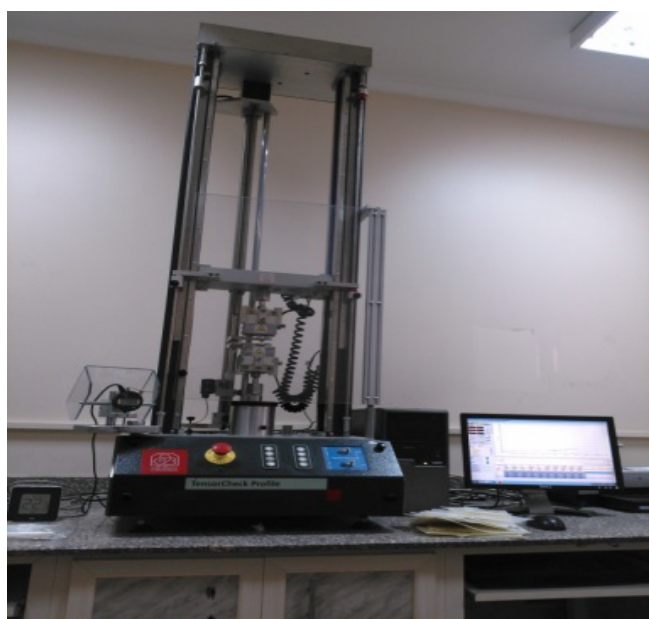
Figure 7: Mechanical measurements tester, (BS EN 60811).
