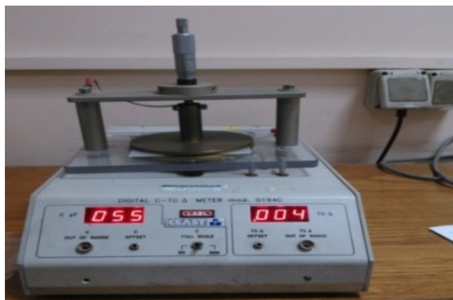
Figure 6: Capacitance tester (ASTM-D150), with two sputtered electrodes.
