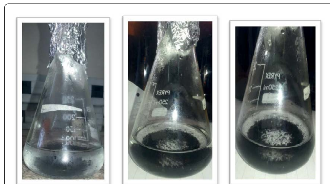
Figure 2: The Progress of Oxidation of MWCNTs using H_2O_2 30% (from left to right).
