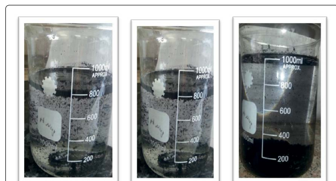
Figure 1: The Progress of Oxidation of MWCNTs using HNO_3 69.7% (from left to right).
