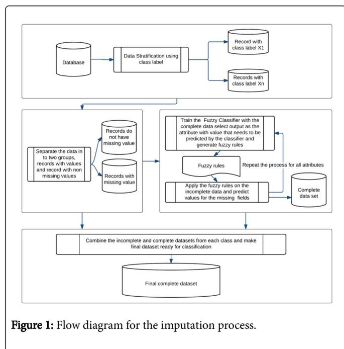
Figure 1: Flow diagram for the imputation process.
