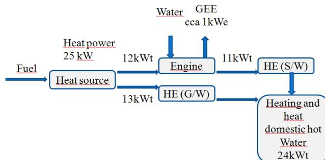
Figure 2: Schema of energy flows in CHP
