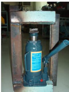
Figure 16: Equipment for pressing stainless tube
