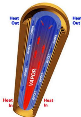
Figure 11: The heat pipe
