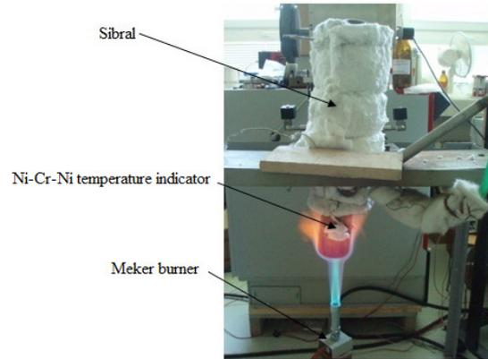
Figure 17: Sodium heat pipe
