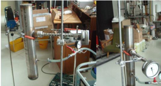
Figure 15: Sodium heat pipe with manometre
