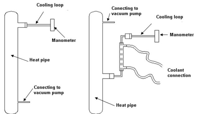
Figure 13: Proposal of pressure measurement in the sodium heat pipe
