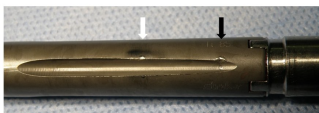
Figure 5: Macroscopic photograph of the lag screw. White arrow indicates the trail by the set screw at the first operation. Black arrow indicates the trail by the set screw made by tightening the set screw before removal. Both trails deviated from the groove.
