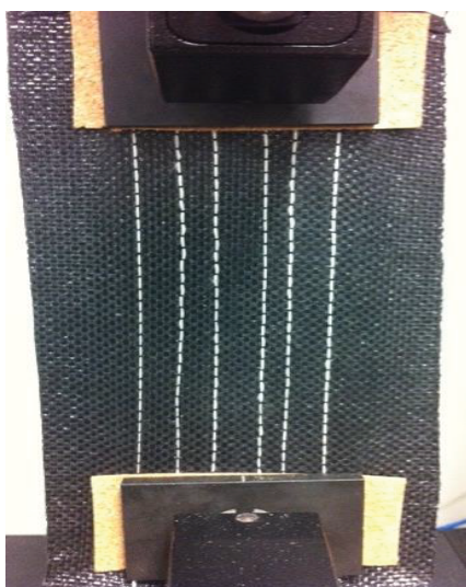
Figure 2: Stitched glass yarn reinforced PE fabric clamped on Instron testing machine.
