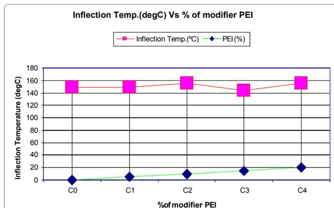
Figure 6D: Line chart for Inflection Temp. (°C) Vs Percentage of modifier PEI
