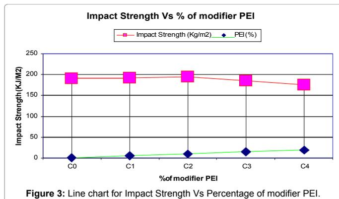
Figure 3: Line chart for Impact Strength Vs Percentage of modifier PEI.
