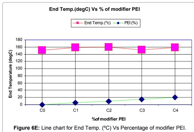
Figure 6E: Line chart for End Temp. (°C) Vs Percentage of modifier PEI.
