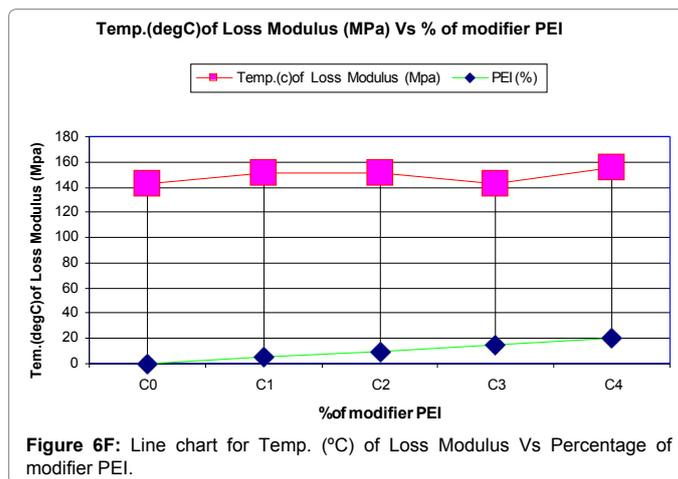
Figure 6F: Line chart for Temp. (°C) of Loss Modulus Vs Percentage of modifier PEI.
