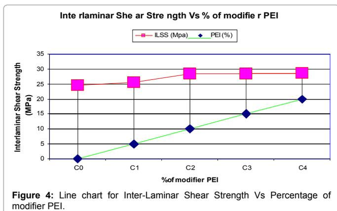
Figure 4: Line chart for Inter-Laminar Shear Strength Vs Percentage of modifier PEI.
