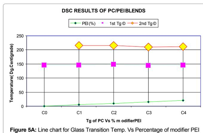
Figure 5A: Line chart for Glass Transition Temp. Vs Percentage of modifier PEI
