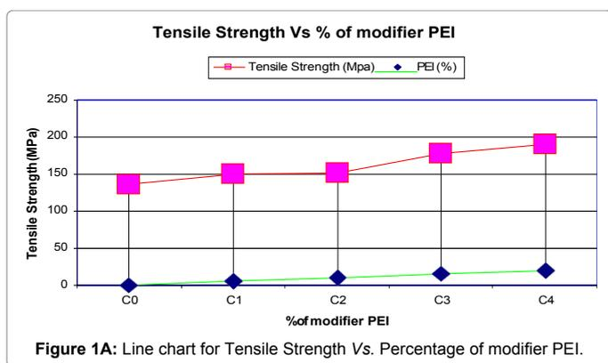
Figure 1A: Line chart for Tensile Strength Vs. Percentage of modifier PEI.
