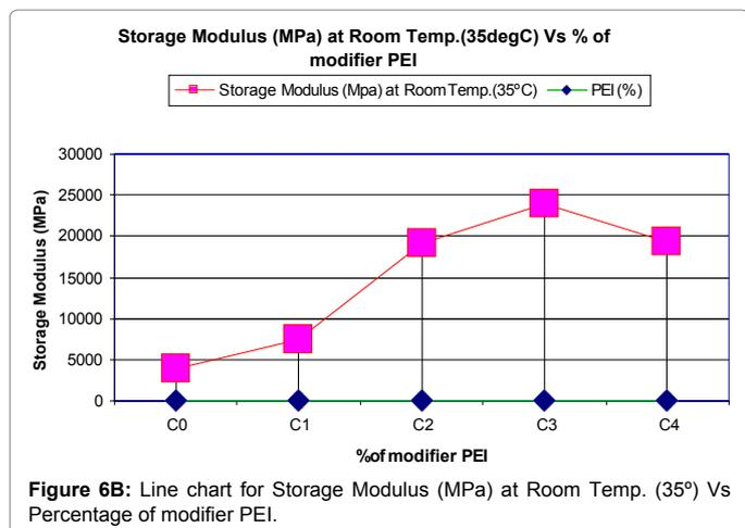
Figure 6B: Line chart for Storage Modulus (MPa) at Room Temp. (35°) Vs Percentage of modifier PEI.
