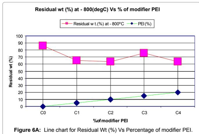
Figure 6A: Line chart for Residual Wt (%) Vs Percentage of modifier PEI.
