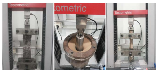
Figure 3: Grab tensile response, Trapezoidal tear strength, CBR puncture strength.
