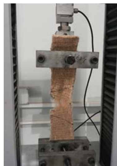
Figure 14: Supporting thread specimen during tear test.
