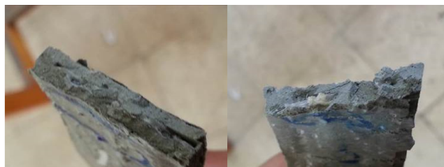
Figure 15: Pultruded jute cement composite failure.
