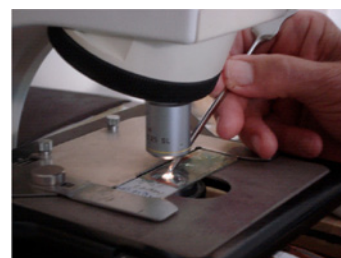
Figure 2: The procedure. Application of pressure on the coverslip under microscopic observation.
