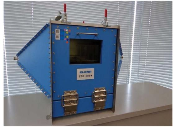
Figure 10. TEM cell for calibration of optical E-field sensor (OES).
