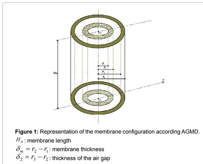
**Figure 1:** Representation of the membrane configuration according AGMD.
