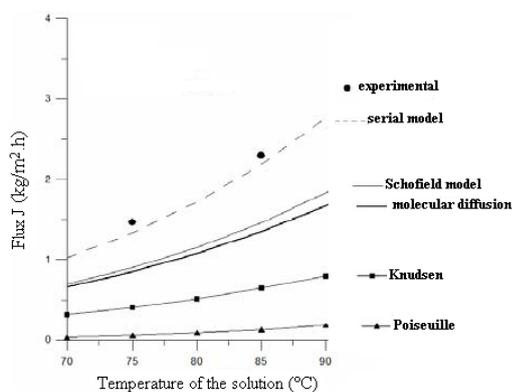
**Figure 16:** Comparison of transfer mechanisms with experimental results for pore radius  $r_p = 25$  nm.
