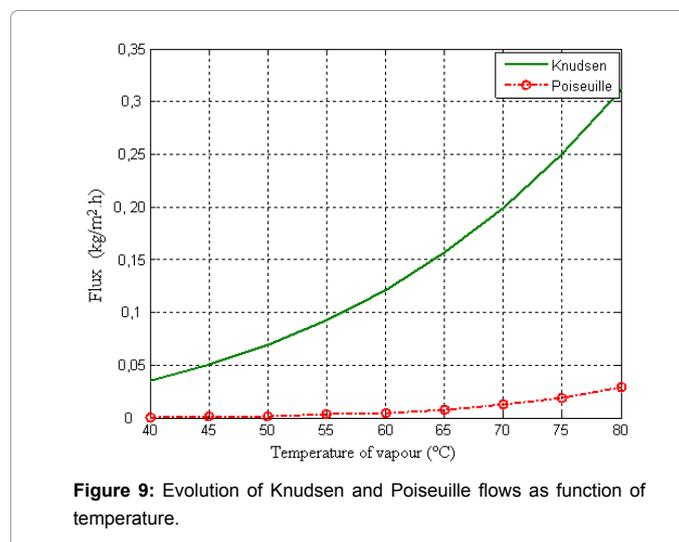
Figure 9: Evolution of Knudsen and Poiseuille flows as function of temperature.
