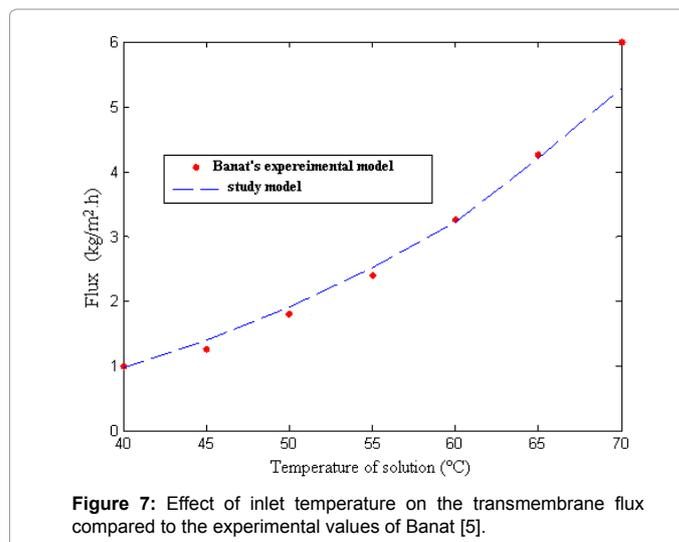
Figure 7: Effect of inlet temperature on the transmembrane flux compared to the experimental values of Banat [5].
