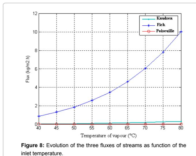
Figure 8: Evolution of the three fluxes of streams as function of the inlet temperature.
