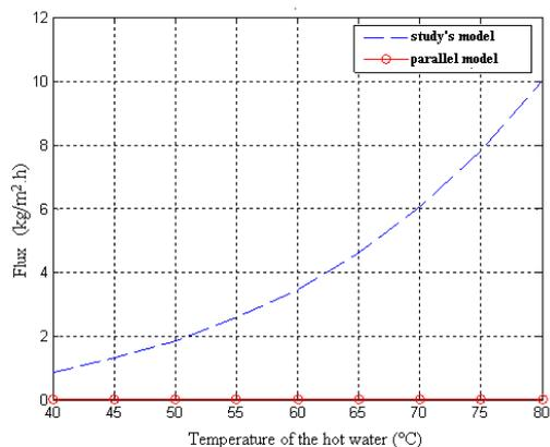
**Figure 15:** Evolution of the molecular flow and model in parallel as function of inlet temperature.
