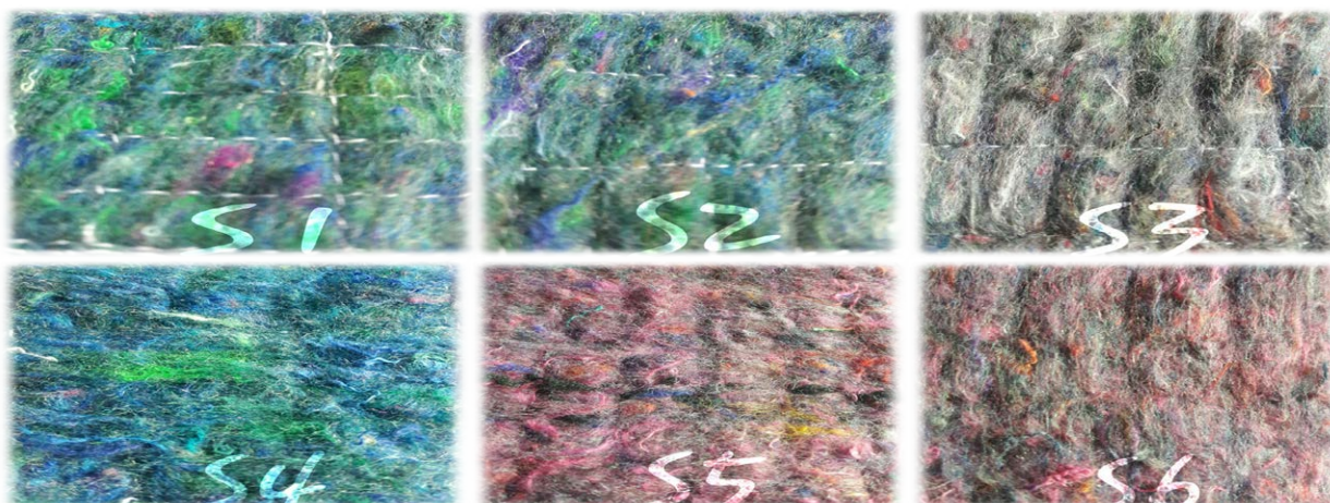
Figure 4: Manufactured stitch bonded nonwoven samples from reclaimed fiber.
