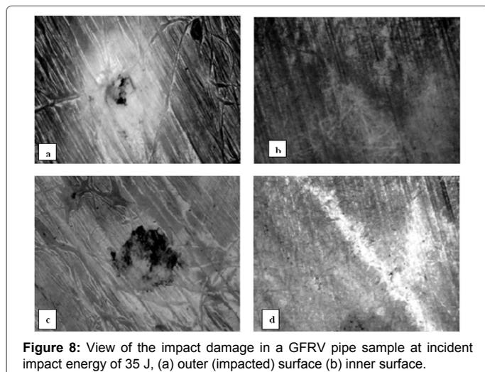
**Figure 8:** View of the impact damage in a GFRV pipe sample at incident impact energy of 35 J, (a) outer (impacted) surface (b) inner surface.
