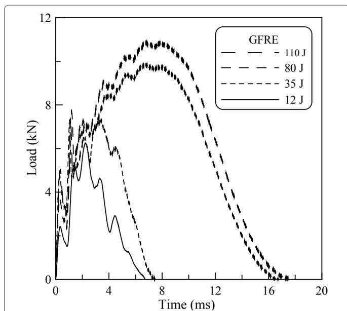
Figure 5: Load-Time traces for GFRE at impact energies of 12, 35, 80 and 110 J.
