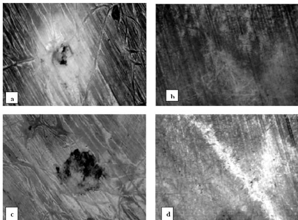
**Figure 8:** View of the impact damage in a GFRV pipe sample at incident impact energy of 35 J, (a) outer (impacted) surface (b) inner surface.
