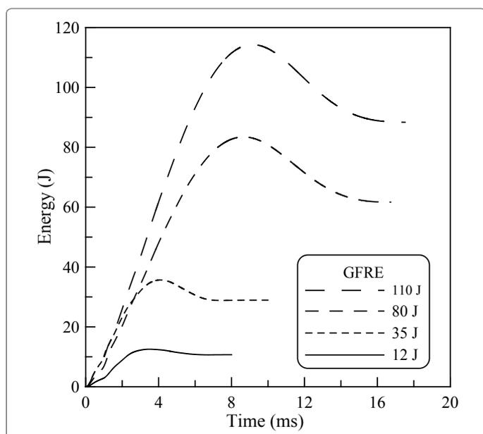
Figure 6: Energy -Time traces for GFRE at impact energies of 12, 35, 80 and 110 J.
