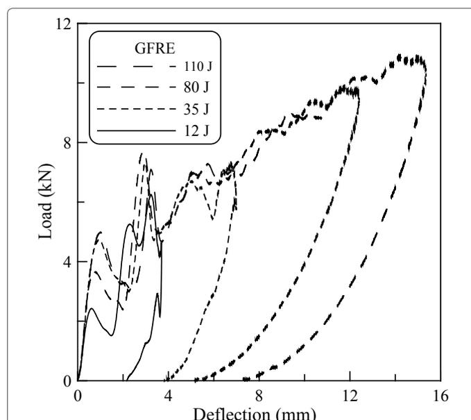
Figure 7: Load -deflection traces for GFRE at impact energies of 12, 35, 80 and 110 J.
