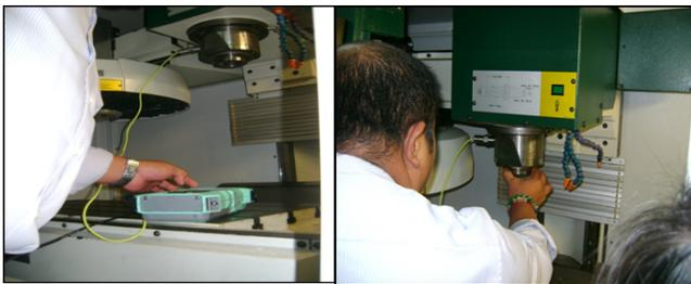
Figure 9: To measure the vibration of CNC Spindle.
