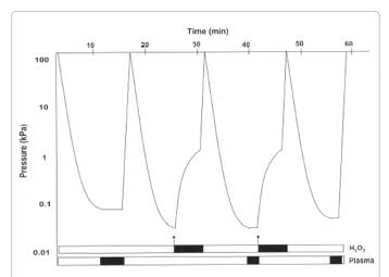
**Figure 1:** The Sterad 100S sterilization cycles. The exposure time, for this particular cycle is about 55 min. Pressure changes during the cycle are shown in a  $\log_{10}$  scale. During the cycle, exposures to hydrogen peroxide gas (injection of gas indicated by arrows) and times of plasma generation are shown (black bars). Note that atmospheric pressure is 760 mmHg.
