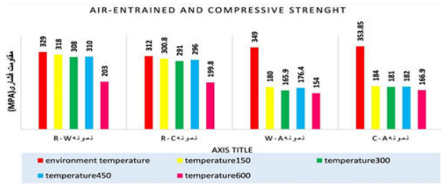
Figure 3. Effect of aeration on the compressive strength of the samples after applying heat.
