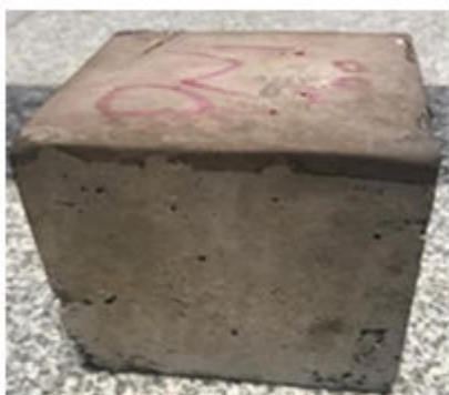
Figure 7. Color changes of the samples after heating.
