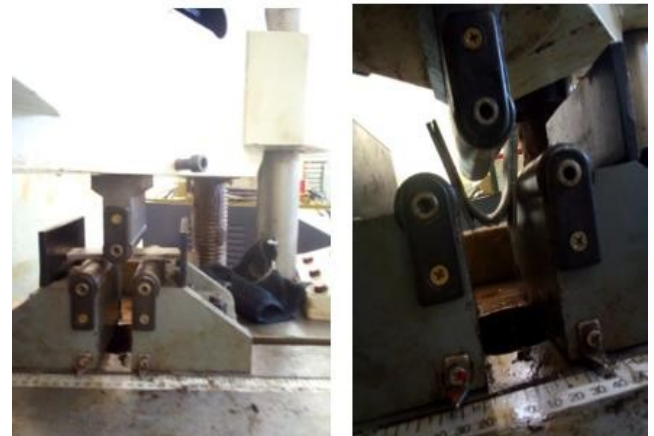
Figure 12. Experimental setup of flexural strength test on UTM machine.
