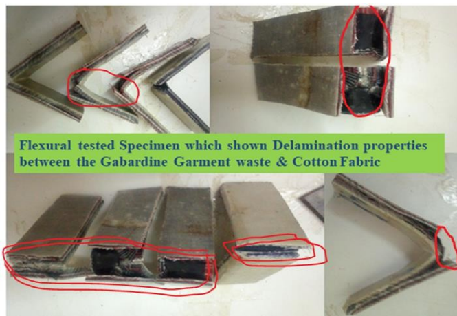
Figure 15. Effects of the reinforcing arrangement and lamination on the delamination properties.
