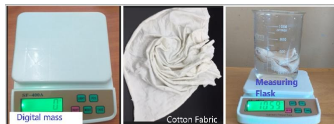
Figure 6. Determination of particle density of the new forming composite based on the principles of Archimedes.
