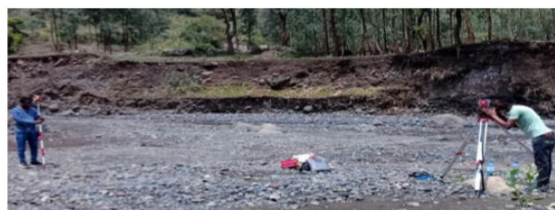
Figure 4. A photo shows surveying the river cross-section.
