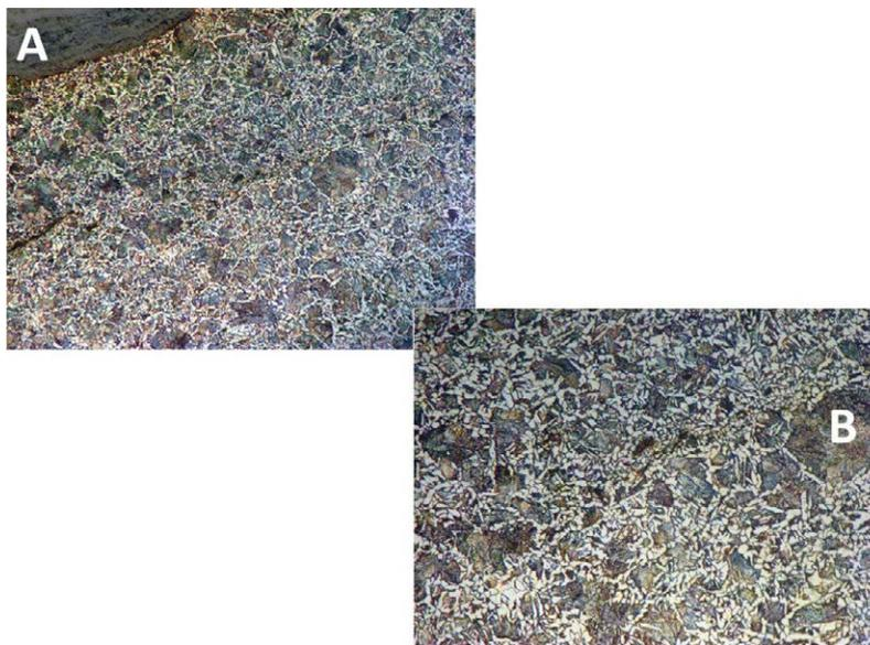
**Figure 5:** A) Micrography obtained by Conventional Optical Microscopy, from the area of the steel nail with a high carbon content. B) Detail at higher magnifications.
