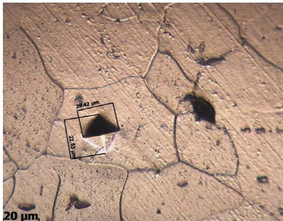
Figure 8: Micrography obtained by Conventional Optical Microscopy, from one of the fingerprints obtained with the Vickers micrometer, with a load of 25 grams.
