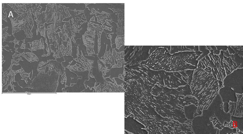
**Figure 6:** A) Micrograph obtained by M.E.B., where it is observed the perlite colony with sheets of prismatic linguistic cementite and oriented in all of it. B) Detail at higher magnifications.
