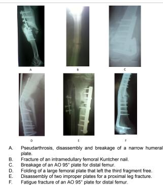
Figure 1: Implants failures.
