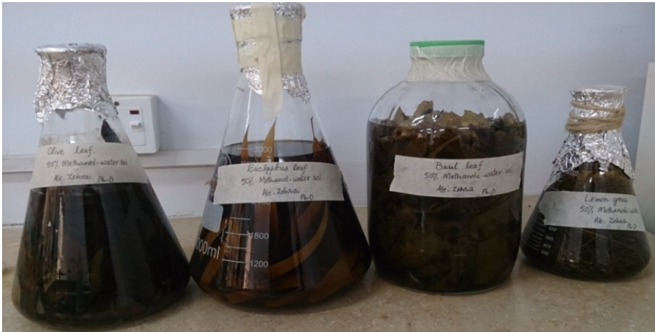
Figure 1: Aerial part (Leaf) of plant soaked in hydro-alcoholic solvent for about 15 days.
