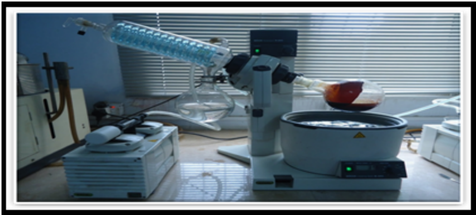
Figure 2: Rotavapor used during the study work showing Olea europaea L. extract to evaporate.
