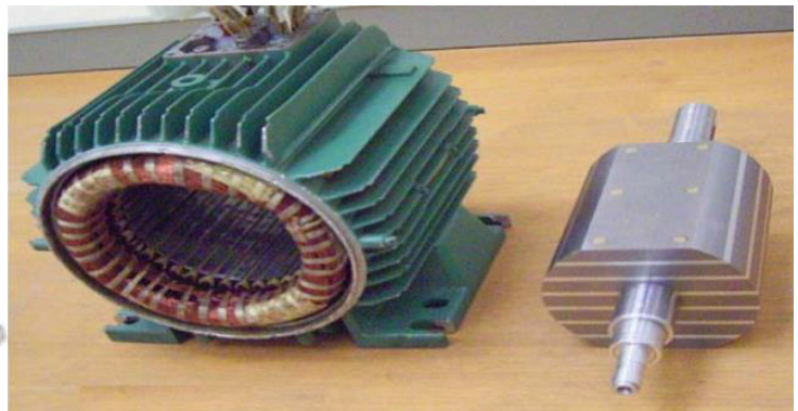
Figure 3: Types of variable reluctance machines; a): Switched Reluctance Machine (SRM); b): Synchronous Reluctance Machine (SynRM).
