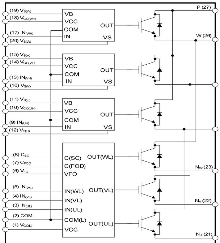
Figure 9: Inner Schematic of FSBS15CH60
