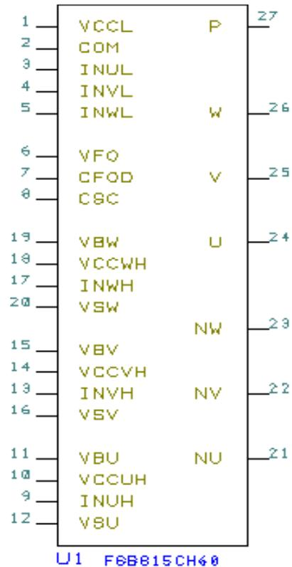
Figure 8: Schematic diagram of SPMTM FSBS15CH60
