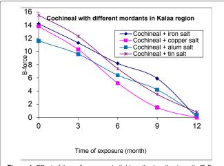
**Figure 1:** Effect of time of exposure to light on the tensile strength (B-Force) of the dyed mordanted wool yarns with Cochineal.
