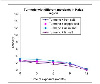
**Figure 5:** Effect of time of exposure to light on the Tenacity of the dyed mordanted wool yarns with Turmeric.
