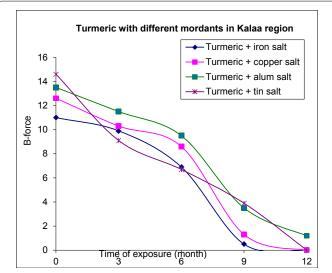
**Figure 2:** Effect of time of exposure to light on the tensile strength (B-Force) of the dyed mordanted wool yarns with Turmeric.
