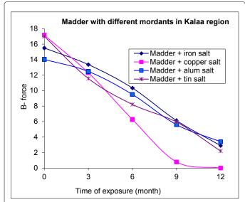
**Figure 3:** Effect of time of exposure to light on the tensile strength (B-Force) of the dyed mordanted wool yarns with Madder.
