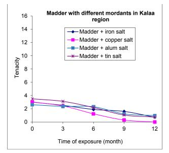
$\textbf{Figure 6:} \ \, \textbf{Effect of time of exposure to light on the Tenacity of the dyed mordanted wool yarns with Madder.}$
