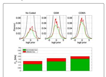
**Figure 8:** APE-plot for various speech conditions in GSM and CDMA networks at SNR = 15 dB and 10-15% frame loss. The Background set contained medium-quality coded speech (i.e., matched scenario).
