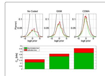
Figure 9: APE-plot for various speech conditions in GSM and CDMA networks at SNR = 15 dB and 10-15% frame loss. The Background set contained un-coded speech (i.e., mismatched scenario).
