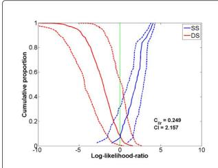
**Figure 6:** Tippett plot showing the FVC performance of medium-quality speech from the CDMA network. The original speech files were corrupted with babble noise at SNR = 15 dB and 10-15% frame loss. The Background set contained medium-quality coded speech (i.e., matched scenario).
