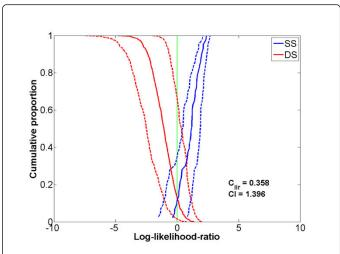
**Figure 7:** Tippett plot showing the FVC performance of medium quality speech from the CDMA network. The original speech files were corrupted with babble noise at SNR =  $15~\mathrm{dB}$  and 10-15% frame loss. The Background set contained un-coded speech (i.e., mismatched scenario).
