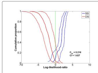
**Figure 5:** Tippett plot showing the FVC performance of medium quality speech from the GSM network. The original speech files were corrupted with babble noise at SNR = 15 dB and 10-15% frame loss. The Background set contained medium-quality coded speech (i.e., matched scenario).
