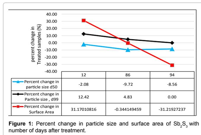
Figure 1: Percent change in particle size and surface area of  $\text{Sb}_2\text{S}_3$  with number of days after treatment.
