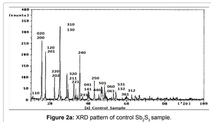
Figure 2a: XRD pattern of control  $\text{Sb}_2\text{S}_3$  sample.
