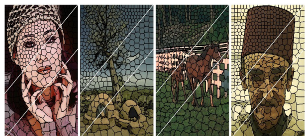
Figure 2: Images segmented into 1000/500/200 super pixels using the proposed LSC algorithm.
