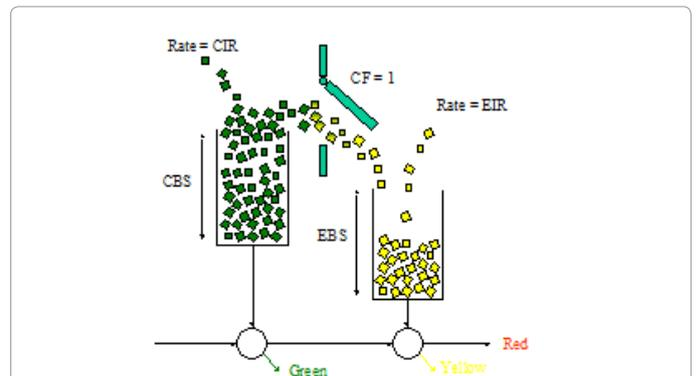
**Figure 3:** Policer behaviour of two buckets EBS and CBS are continuously filled in at a rate EIR and CIR respectively.
