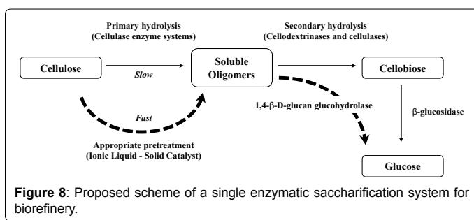
**Figure 8:** Proposed scheme of a single enzymatic saccharification system for biorefinery.
