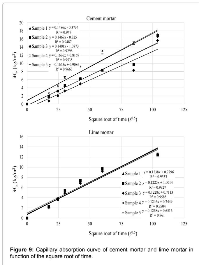
Figure 9: Capillary absorption curve of cement mortar and lime mortar in function of the square root of time.
