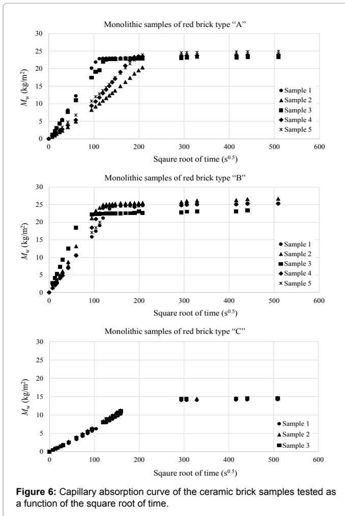
bricks "A" and "C" are greater than the density of the ceramic brick type "B". The experimental results obtained are in accordance with other experimental values found in literature, i.e., several authors presented a range of experimental values between 0.05 and 0.29 kg/m<sup>2</sup>s<sup>0.5</sup>, for these building materials [20-23].
