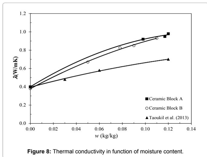
Figure 8: Thermal conductivity in function of moisture content.
