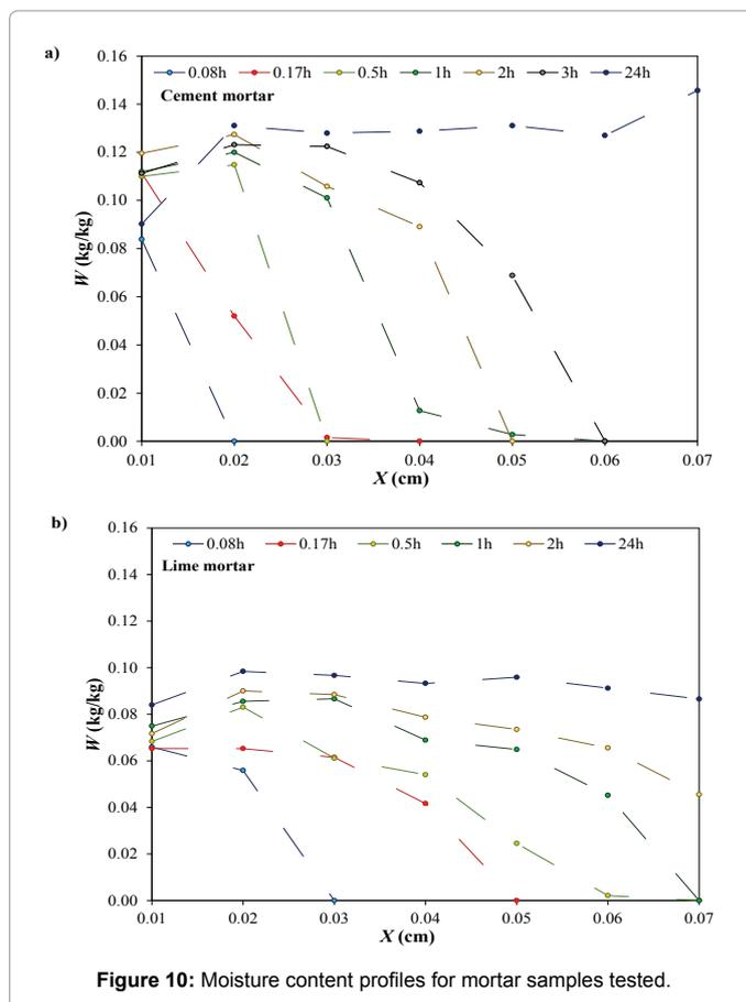
Figure 10: Moisture content profiles for mortar samples tested.
