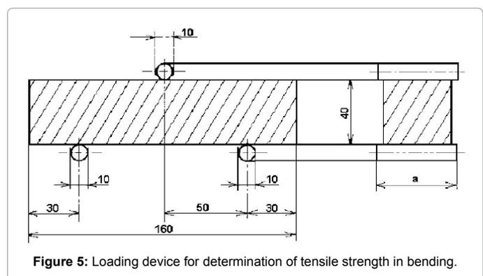
Figure 5: Loading device for determination of tensile strength in bending.
