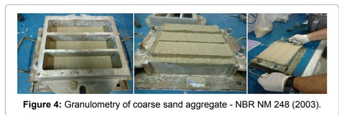
Figure 4: Granulometry of coarse sand aggregate - NBR NM 248 (2003).
