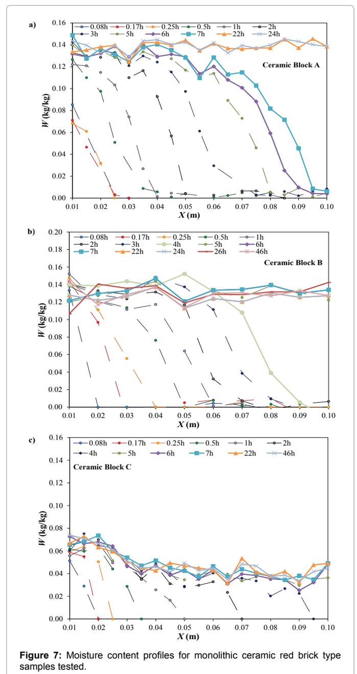
**Figure 7:** Moisture content profiles for monolithic ceramic red brick type samples tested.
