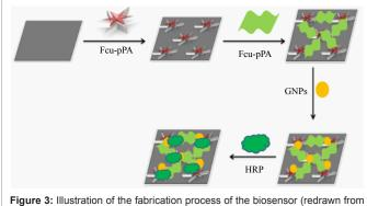
Figure 3: Illustration of the fabrication process of the biosensor (redrawn from reference [52], [80]).
