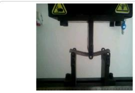
Figure 3: Flexural strength set-up.
