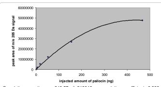
Correlation equation: y=-248.57 x<sup>2</sup>+218318 x; correlation coefficient: 0.998, where y is the peak area, x is the injected amount in ng. Chromatographic conditions — Column: ZIC-pHILIC (150 mm × 4.6 mm I.D., d\_ 5 µm); mobile phase: MeCN - 40 mmol formate buffer (pH 3.5) 80:20 v/v; flow rate: 0.5 ml/min; temperature: 40°C; injection volumes: 1 µl, detection ESI (+ mode): MS, scan range 40 Da to 400 Da.
