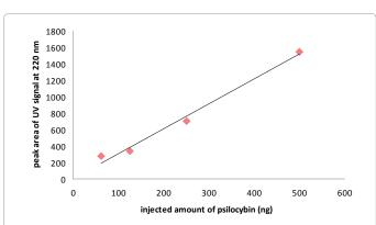
Correlation equation: y=3.0464 x; correlation coefficient: 0.993, where y is the peak area, x is the injected amount in ng. Chromatographic conditions — Column: ZIC-pHILIC (150 mm × 4.6 mm I.D., d<sub>p</sub> 5 µm); mobile phase: MeCN - 40 mmol formate buffer (pH 3.5) 80:20 v/v; flow rate: 0.5 ml/min; temperature: 40°C; injection volumes: 1 µl, UV photometric detection at 220 nm.
