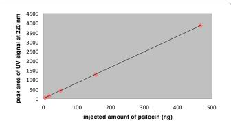
Correlation equation: y=8.2746 x; correlation coefficient: 0.999, where y is the peak area, x is the injected amount in ng. Chromatographic conditions — Column: ZIC-pHILIC (150 mm × 4.6 mm I.D., d<sub>p</sub> 5 µm); mobile phase: MeCN - 40 mmol formate buffer (pH 3.5) 80:20 v/v; flow rate: 0.5 ml/min; temperature: 40°C; injection volumes: 1 µl, UV photometric detection at 220 nm.
