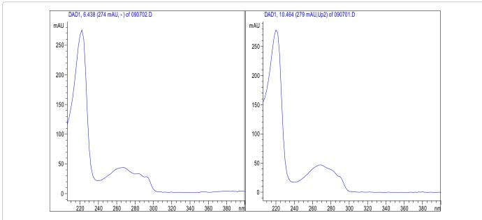
Chromatographic conditions — Column: ZIC-pHILIC (150 mm × 4.6 mm I.D.,  $d_p 5 \mu m$ ); mobile phase: MeCN - 40 mmol formate buffer (pH 3.5) 80:20 v/v; flow rate: 0.5 ml/min; temperature: 40°C; injection volumes: 1  $\mu$ l, diode array detection in the range of 190 nm to 400 nm.
