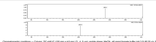
Chromatographic conditions — Column: ZIC-pHILIC (150 mm × 4.6 mm l.D.,  $d_p^{-5} \mu$ m); mobile phase: MeCN - 40 mmol formate buffer (pH 3.5) 80:20 v/v; flow rate: 0.5 ml/min; temperature: 40°C; injection volumes: 1 µl, detection ESI (+ mode): MS, scan range 40 Da to 400 Da.
