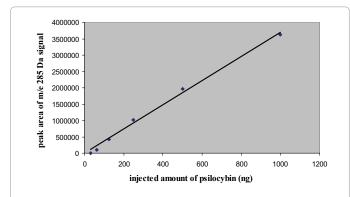
Correlation equation: y=3691.4 x; correlation coefficient: 0.997, where y is the peak area, x is the injected amount in ng. Chromatographic conditions — Column: ZIC-pHILIC (150 mm × 4.6 mm I.D., d<sub>p</sub> 5 µm); mobile phase: MeCN - 40 mmol formate buffer (pH 3.5) 80:20 v/v; flow rate: 0.5 ml/min; temperature: 40°C; injection volumes: 1 µl, detection ESI (+ mode): MS, scan range 40 Da to 400 Da.
