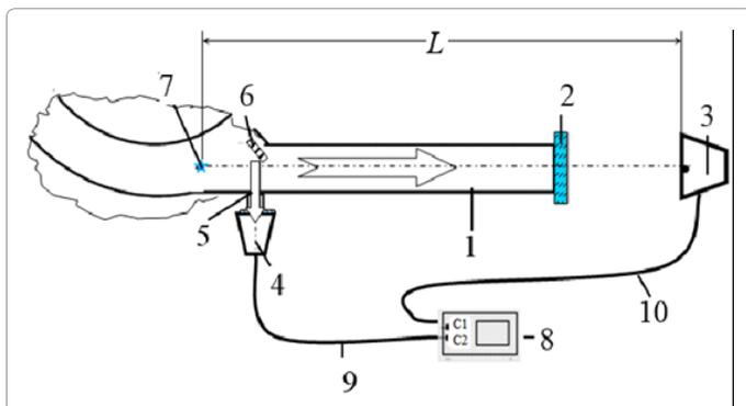
**Figure 2:** Proposed schematic of the measurements: (1) radiation output channel; (2) output window; (3) radiation detector of the measuring channel; (4) detector of the reference channel; (5) reference radiation output channel; (6) mirror of the reference channel output; (7) point of emission of an electron from a stationary orbit; (8) two-beam oscilloscope; (9) reference channel cable; (10) measuring channel cable.
