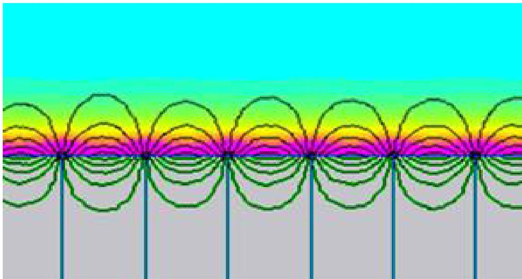
**Figure 4:** Schematic representation of the magnetic field generated by anisotropic NdFeB magnetic strip. Only one side of the strip is highly magnetized (purple color), and magnetic field intensity decreases exponentially with the distance (yellow and green colors). Curved magnetic lines are also represented.
