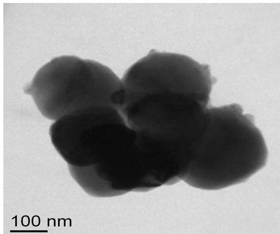
**Figure 2:** Transmission electron microscope (TME) image of iron oxide ( $\text{Fe}_3\text{O}_4$ ) magnetic nanoparticles. The cluster formed as results of sample preparation due to dried environment.
