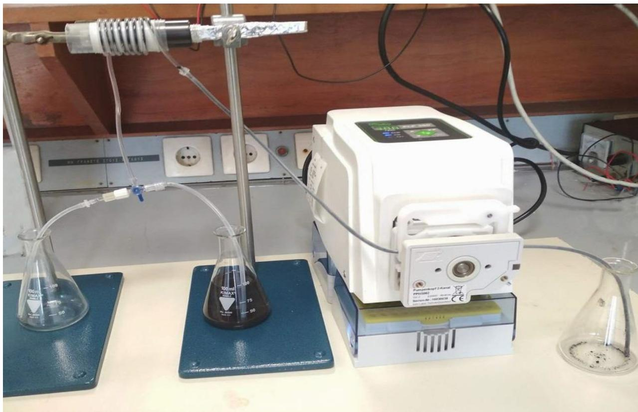
Figure 6: Complete apparatus after magnetic separation. Magnetic particles are trapped on the spiral hose without liquid covering them.
