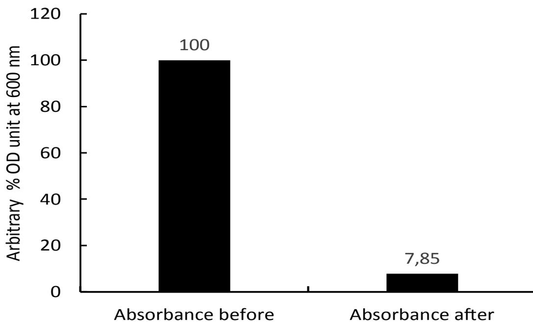
Figure 7: Spectrophotometer analysis of the optical density (OD) of alcoholic solutions before and after magnetic separation measured at light wavelength of 600 nm.
