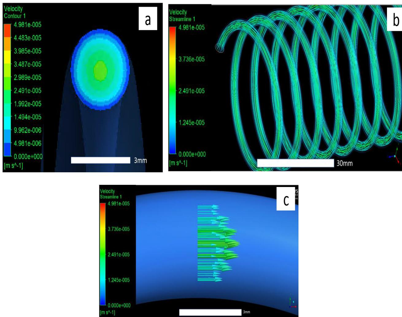
**Figure 3:** (a) cross section view-velocity contours; (b) laminar flow distribution in the spiral hose; (c) lateral view-velocity vectors.
