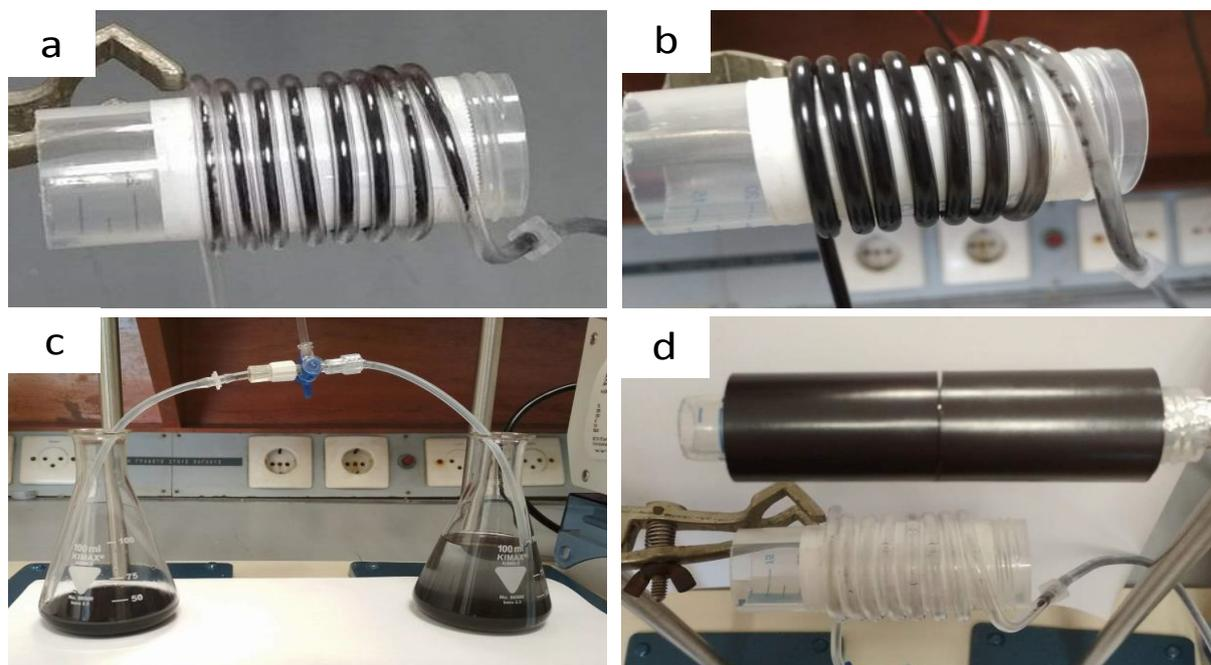
**Figure 8:** (a) magnetic core removal; (b) harvesting of magnetic particles from spiral hose; (c) magnetic particles collection into separate flasks; (d) spiral hose completely clean after magnetic particles harvesting.
