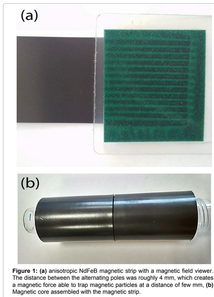
Figure 1: (a) anisotropic NdFeB magnetic strip with a magnetic field viewer. The distance between the alternating poles was roughly 4 mm, which creates a magnetic force able to trap magnetic particles at a distance of few mm, (b) Magnetic core assembled with the magnetic strip.
