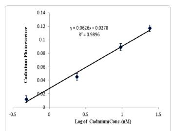
**Figure 4:** Logrithmic relationship of Cadmium (0.5-24 nM) with enzyme activity, in spiked milk sample with acridine orange as the sensing dye (result obtained by applying standard deviation to triplicate experiments).
