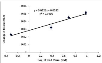
**Figure 2:** Logrithmic relationship of lead concentration with enzyme activity. The Linear range of detection achieved was 0.48-9.66 nM Pb in modified microarray method (result obtained by applying standard deviation to triplicate experiments).
