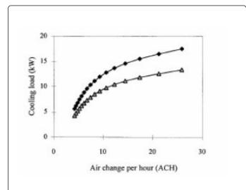
Figure 7: Cooling loads by night ventilation for desired room indoor air temperatures of 23 and 25°C.
