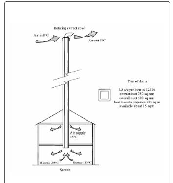
Figure 2: Small house natural ventilation with heat reclaims (a very tall chimney).
