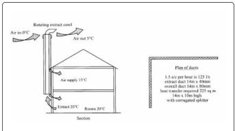
Figure 3: Ventilation duct supply and extract wraps around the building.
