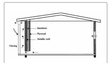
Figure 4: Schematic representations of the passive solar house and natural ventilation by metallic solar wall.
