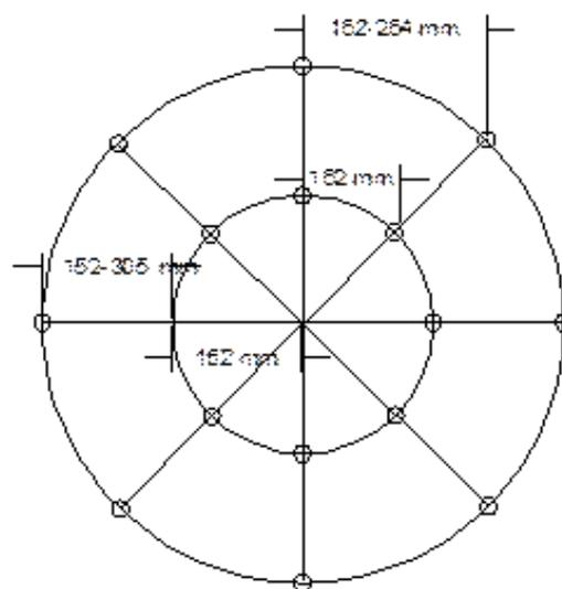
Figure 4: Schematic of air velocity measurement points (smaller circles) across the radius of an exhaust fan.
