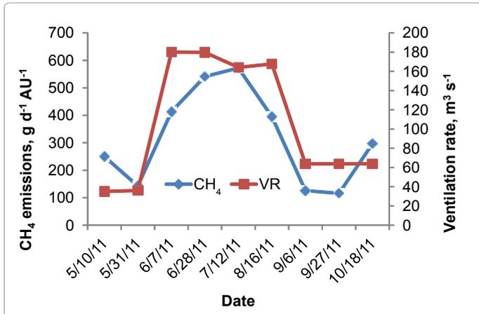
Figure 9: Variation of methane (CH<sub>4</sub>) emissions from deep pit manure storage exhaust fan.
