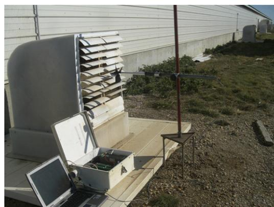
Figure 3: Set-up used for fan calibration using a bi-directional Gill propeller anemometer.
