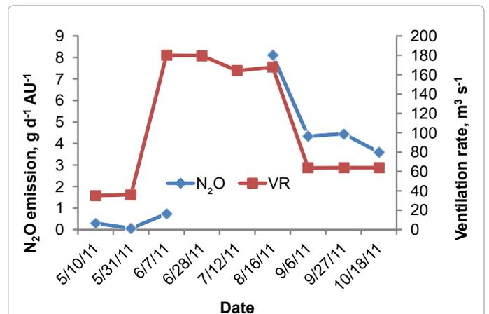
Figure 11: Variation of nitrous oxide (N<sub>2</sub>O) emissions from deep pit manure storage exhaust fan.
