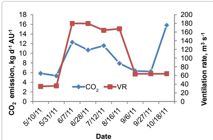
Figure 10: Variation of carbon dioxide (CO<sub>2</sub>) emissions from deep pit manure storage exhaust fan.
