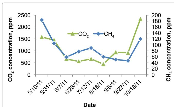
Figure 7: Average methane ( $\text{CH}_4$ ) and carbon dioxide ( $\text{CO}_2$ ) concentration from deep pit manure storage measured in exhaust fan.
