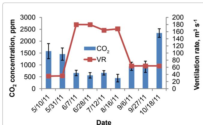
Figure 6: Variation of carbon dioxide ( $\text{CO}_2$ ) concentration from deep pit manure storage measured in exhaust fan. Error bars represent standard deviation.
