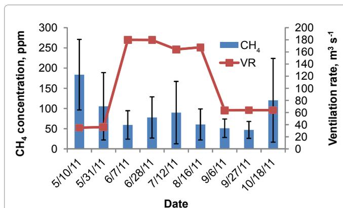
Figure 5: Variation of methane concentration from deep pit manure storage measured in deep pit exhaust fan. Error bars represent standard deviation.
