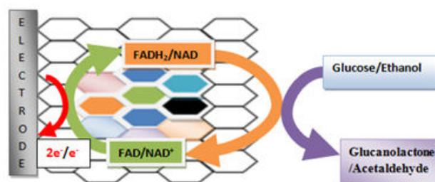
**Figure 1.** Graphen based glucose/ethanol enzymatic biosensor.
