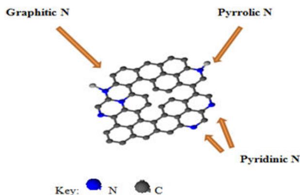
Figure 2. Doping position of N on graphen.
