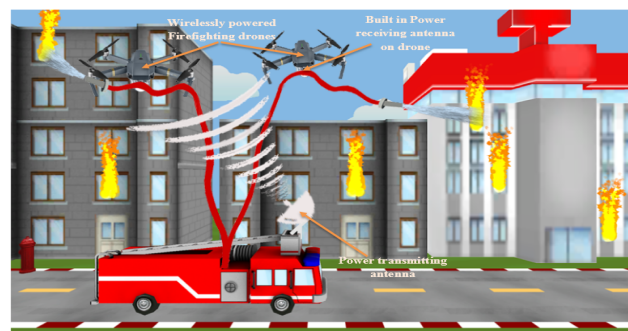
Figure 13: Firefighting drones getting its power wirelessly from firefighting vehicle.
