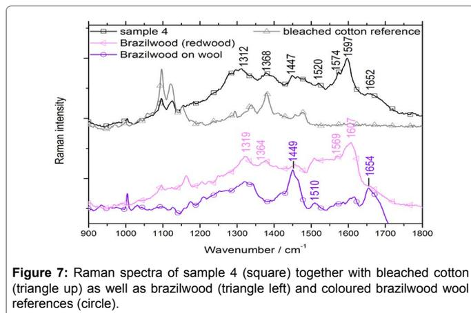
**Figure 7:** Raman spectra of sample 4 (square) together with bleached cotton (triangle up) as well as brazilwood (triangle left) and coloured brazilwood wool references (circle).
