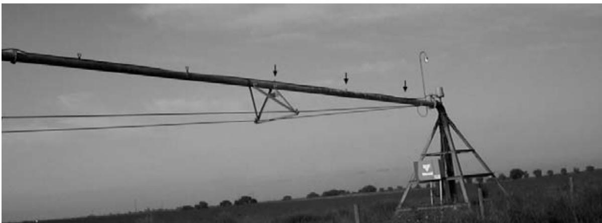
Figure 2: Photo of the center-pivot beginning showing three closed outlets.
